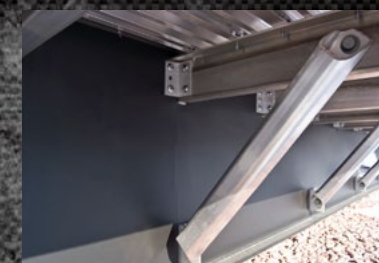
Aluminum knee braces are lighter and longer lasting than steel and will withstand the beating from rocks and road debris.
