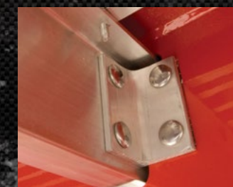
Wilson's aluminum crossbar clips are attached to the main beams and the crossbars using corrosion resistant stainless steel fasteners. A copolymer material is also placed between the aluminum clip and steel beam to insulate the two dissimilar metals. Couple this concept with the insulating properties of the Corsol metal coating and the result is your best defense against electrolysis.
